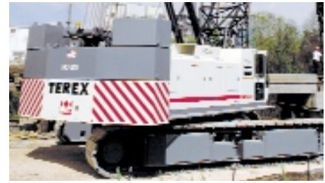
Counterweight hydraulically extends
